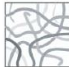
Amorphous polymers - long chains
