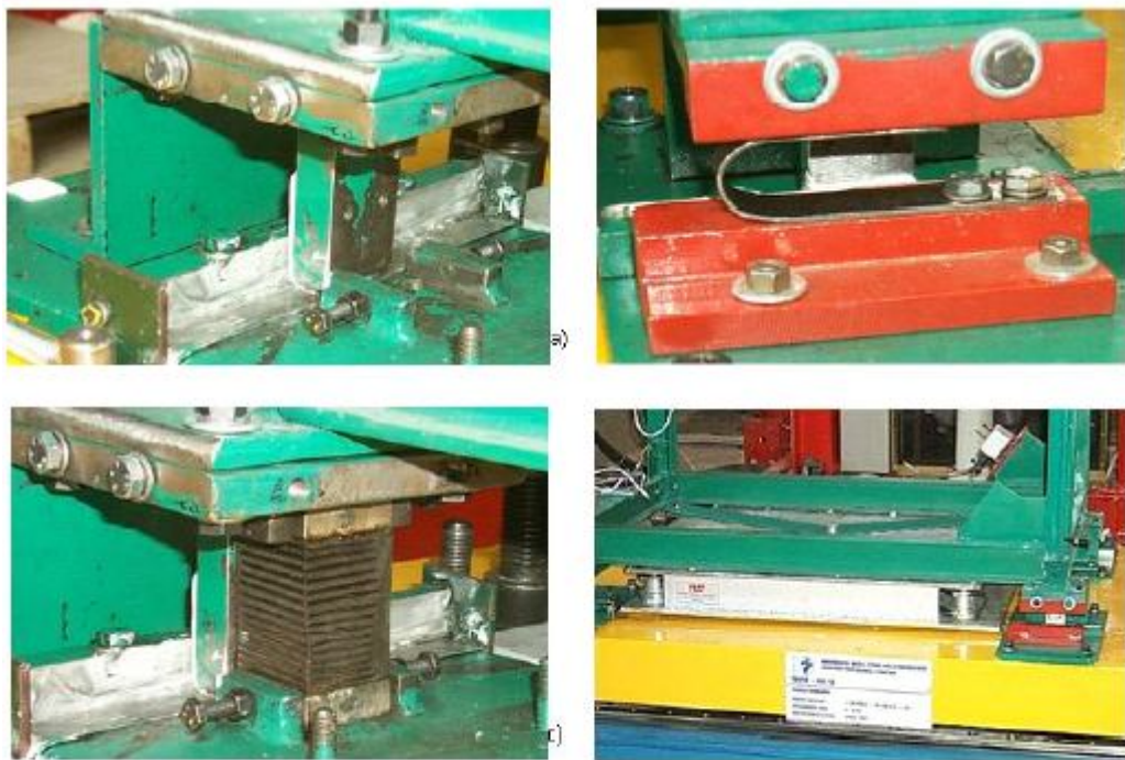
a) Steel-PTFE slider; b) steel based device; c) rubber based device; d) SMA based device
