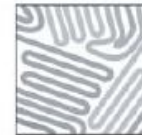
Folded chains (semicrystalline)
